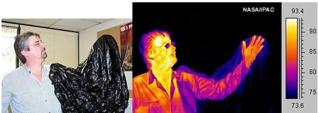
Fig. 9. Some apparent black bodies are not black-bodies: visible vs. infrared opacity. ( http://en.wikipedia.org/ ).
