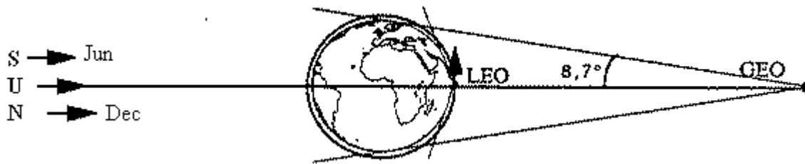
Fig. 1. Relative distances and viewing angles for LEO and GEO.
