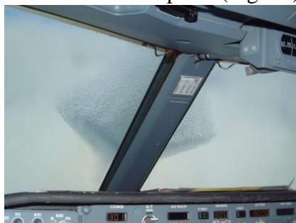
Fig. 11. Severe icing on the central windscreen pillar of an aircraft, formed in under a minute flying at 6 km altitude (FL200).
