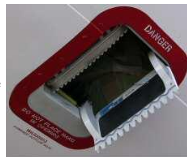
Fig. 2. Cabin pressure regulation as a function of altitude, and a photo of an outflow valve (below the fuselage) that regulates it.
