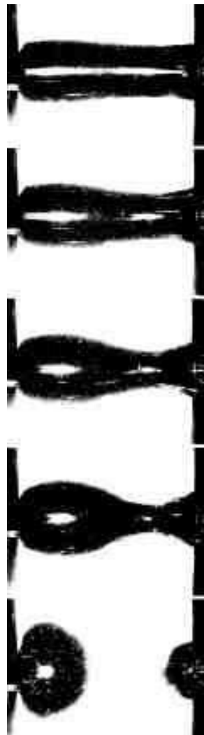
Fig. 2. Breaking sequence of a 100 mm long liquid column. Times to the last one, are 0, -2, -4, -10, and -50 s.
