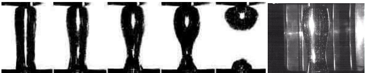
Fig. 5. Film pictures of the breaking sequence of a 100 mm long liquid column in Spacelab-D1-FLIZ experiment (times, relative to the last one, are 0, -2, -4, -10, and -50 s). Notice the difficulties for accurate edge detection in the liquid bridge because of the bright background (the video frame with less contrast shown last is even worse for the purpose).
