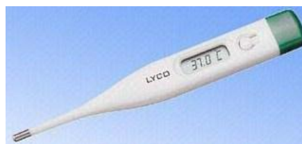
Fig. 5. An example of thermistor application: digital clinic thermometer.
