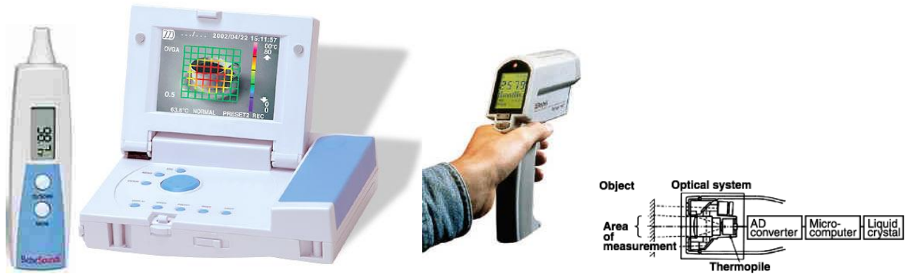
Fig. 6. Ear IR-thermometer, 2-D array IR-unit, handheld industrial IR-unit, and some internal details.
