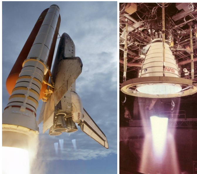
Fig. 4. Shock diamonds (blue cones) in Shuttle's main engine nozzles during STS-120 launch ( NASA ), and during tests.
