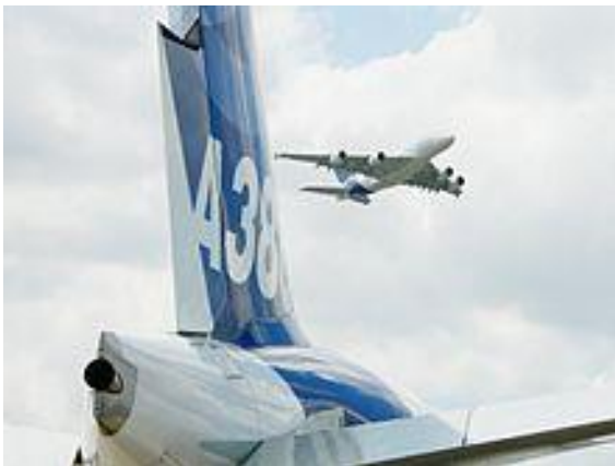
Fig. 11. a) The APU exhaust at the tail end of an A380 . b) B787 Dreamliner APU.
