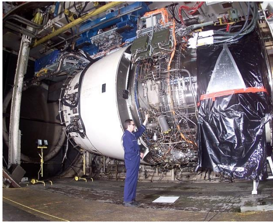
Fig. 13. Overhauling on a RR-Trent-900 jet engine ( Wiki ).
