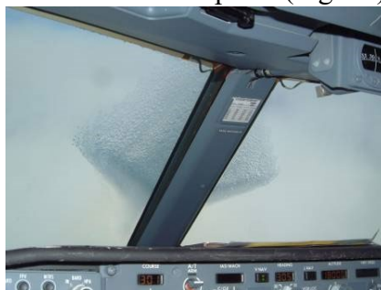
Fig. 11. Severe icing on the central windscreen pillar of an aircraft, formed in under a minute flying at 6 km altitude (FL200).
