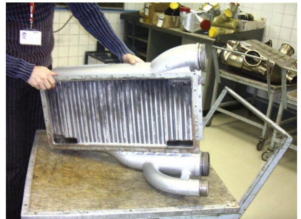
Fig. 8. ECS heat-exchanger layout (typical size of each HE is 0.7 \cdot 0.5 \cdot 0.3 \text{ m}^3 , and 10..15 kg). Photography of one of the heat exchangers.
