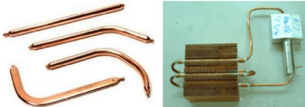
Fig. 6. a) Four traditional or stick heat pipe (SHP); the evaporator and condenser zones can be anywhere. b) Loop heat pipe (LHP), with fins at the condenser zone; the evaporator is the white hand-written piece, and the compensation chamber is the metal bright adjacent element. ( China-heatpipe.net ).
